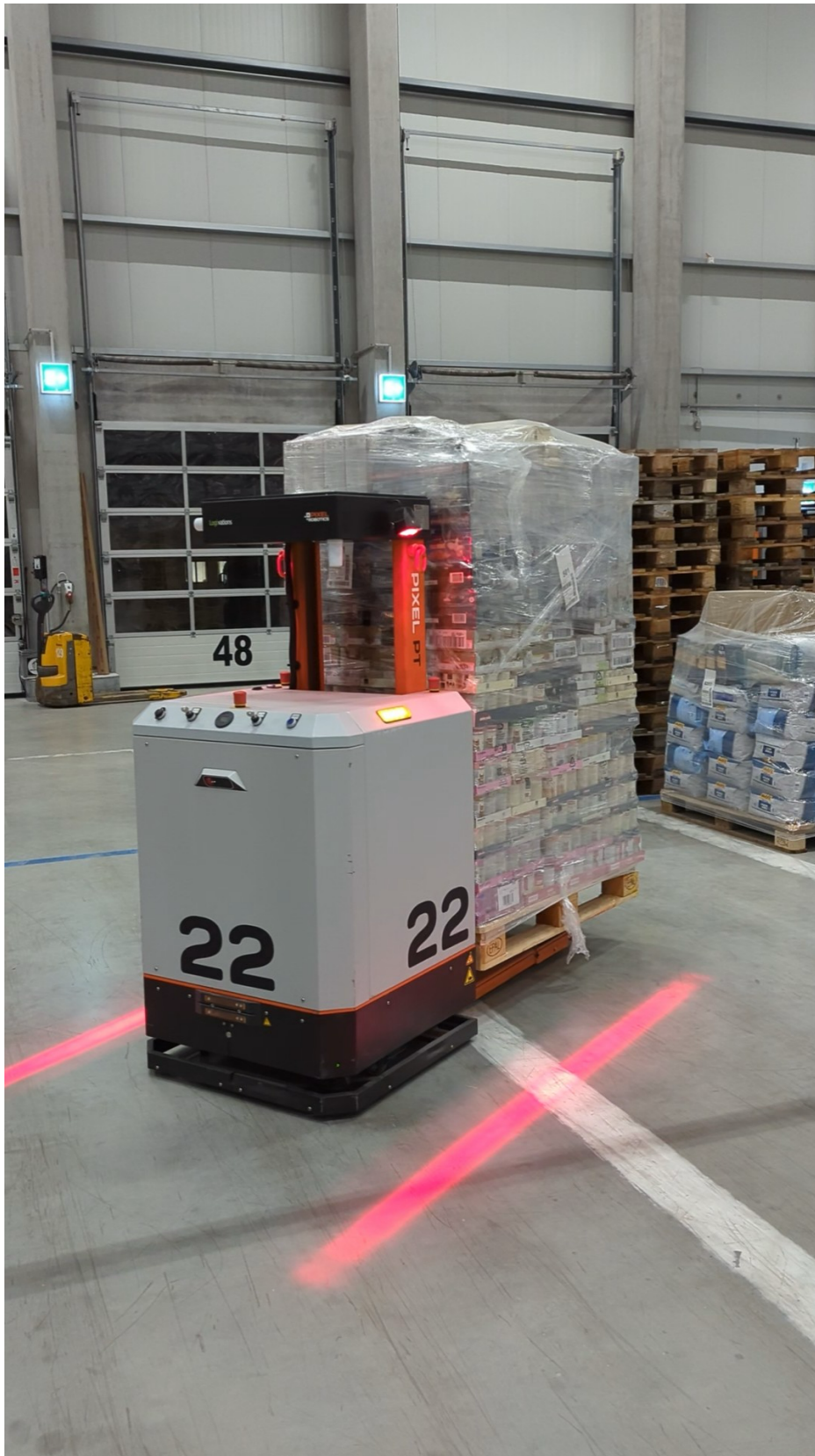
Pic 1: AI Transport Robots: Navigating with Foil in the Safety Scanner's Field of View (Source: Pixel Robotics)
